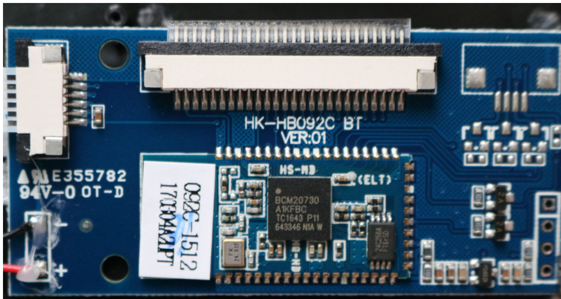
Figure 4: PCB of the tested 1byone wireless keyboard with BCM20730 Bluetooth transceiver and EEPROM chip
